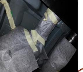
Wrap and tape off transmission, transfer case, propeller shaft, cables, wiring, exhaust, etc.to protect from overspray as illustrated above.
