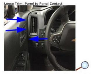
An interface may cause a rattle or buzz (for example, between a door and instrument panel).
