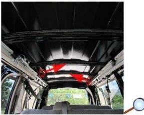
2. Locate the third and fourth roof bow (counting from the front of the vehicle).
