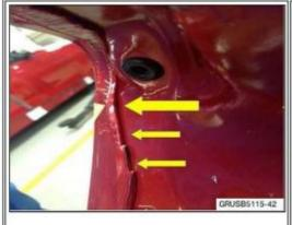
Do not remove the existing PVC seal and only apply PVC sealer to the wavy area.
