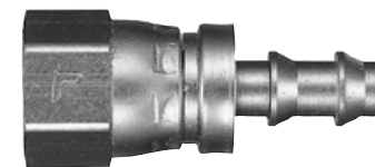
Universal Female Swivel 1/4 Hose I.D., 1/2-20 Thread Size
