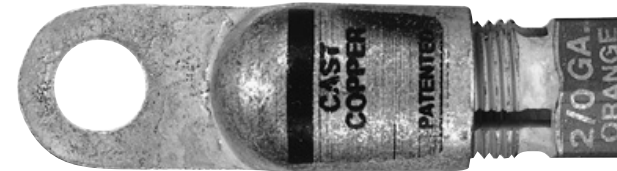
Starter/Cable Lug 2/0 Ga., 3/8 Stud Orange Color Code
