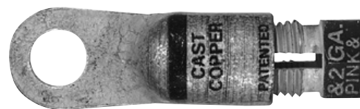
Starter/Cable Lug 1 and 2 Ga., 3/8 Stud Green Color Code
