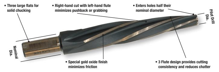
Lawson's Regency® Tapered Reamers are an ideal solution for hole enlargement and aligning misaligned holes on fleet trailers, truck frames, or other steel construction applications.
