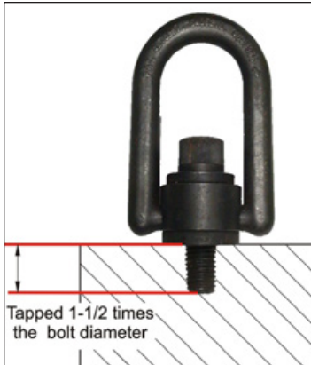
Swivel hoist ring in threaded hole
