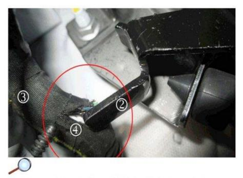
Note: Photograph shows a damaged (4) body wire harness. Note the contact between the park brake pedal assembly switch activating tab (2) and the body wire harness (3).
