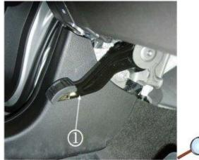
Locate the park brake pedal assembly (1). The park brake pedal assembly is located under the instrument panel on the driver side of the vehicle.
