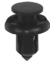
Front Bumper Push-Type Retainer 20mm Head Dia., 13mm Stem Length Fits into 10mm Hole
