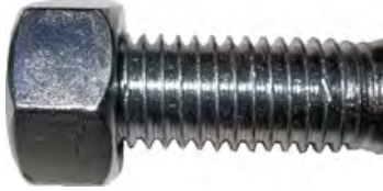
Nicked thread on cap screw interfering with hex nut.
