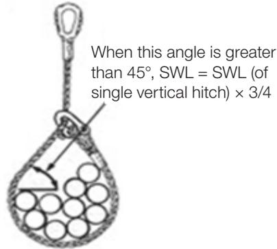
**Angle of choke is less than 45°**
