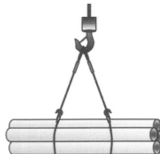
When using two choker hitches, the hook openings should face out from the center of the load.
