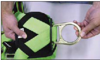
Testing the D-rings
